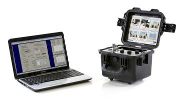
The Portable Accelerometer Calibration System, Model K9145D10, features accurate back-to-back comparison calibration of accelerometers in accordance with ISO 16063-21 (2003). A derivative of the industry-leading 9155 Accelerometer Calibration Workstation and based on a laptop PC system with a state-of-the-art 24-bit USB dynamic signal analyzer module, the K9145D10 offers a portable, turnkey calibration solution suitable for both laboratory and field portability.
