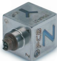
356A32 - Triaxial ± 50 g pk, Sensitivity 100 mV/g
