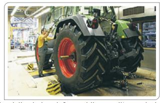
Specially designed for end-line quality- and check-out tests. Two vehicles can be tested simultaneously on the combination "two-axle function roller test stand and brake roller test stand
