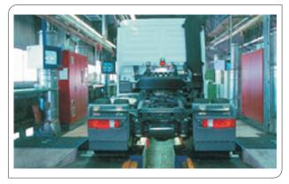
Vehicle component diagnosis by using a variety of selectable test programs
