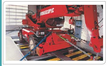
Expensive test drives on the road are no longer needed, but can be simulated on a test stand providing reproducible results independent of weather conditions.
