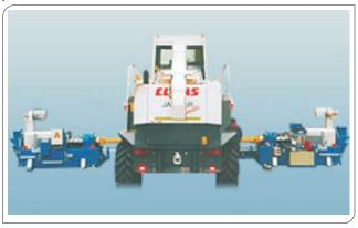
The test stand essentially consists of two self-aligning AC motor units.
