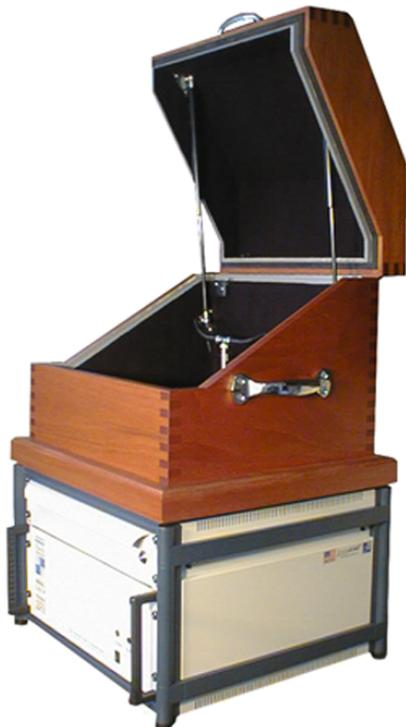
The Precision Acoustic Calibration Workstation Model 9350C is an automated, accurate, turnkey, PC-based system that features cost-effective calibration of 1/8 in, 1/4 in, 1/2 in and 1 in microphone cartridges (open-circuit sensitivity), microphone cartridges with preamplifiers (closed-circuit sensitivity), as well as microphone Frequency Response Function.
